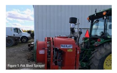
The sprayer uses a Pak Blast Sprayer mounted on the back of a tractor using a 3 point hitch and uses a Smart Guided Systems controller to detect foliage and articulate spray nozzles to apply product to plant tissue.
